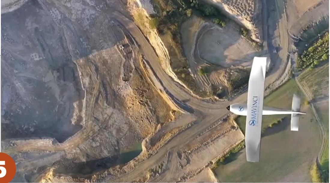
MAVinci autonomous micro air-vehicle surveys an open mining site.
